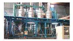
To enhance the luster and strength of its fabrics, Zaber and Zubair (Z&Z) Fabrics Limited of Noman Group, apply a mercerization technique where the fabric is treated with caustic soda (NaOH) and other wetting agents. At the end of the process, the mercerized fabric is rinsed with water to remove the excess caustic.
