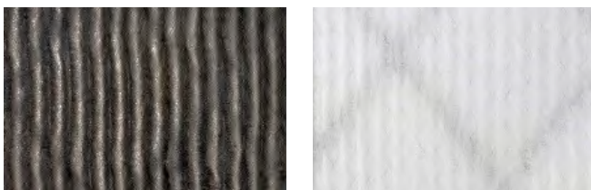
Dirty and clean air filter
