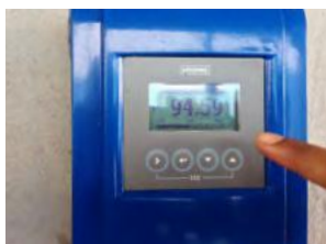
Installation of water flow meter in the waste water line of an audited mill
