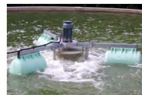
Vertical axis floating agitation/aeration system
